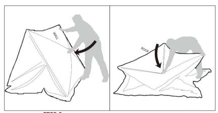
**STEP 2**: Using your hand, push the center hub in on each of the walls until they collapse inward. Shelter will fall to the ice on its own. Push in the roof hub until it collapses as well.
