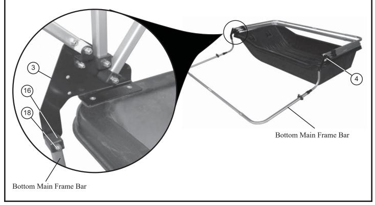
13. Set up main frame bars by grasping with both hands and pushing upward until button clicks into place. Start with bottom main frame bar and continue to the back main frame bar pushing lengthened bars into appropriate position.
