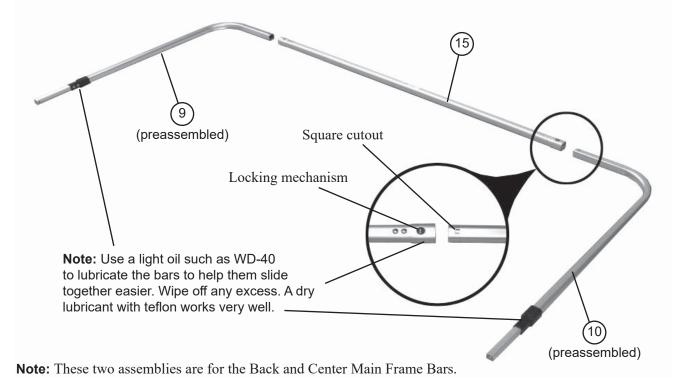
6. Position middle main frame (Item 15), left side front elbow and extension (Item 11), and right side front elbow and extension (Item 12) as shown. Align locking mechanism in item 15 with square cutout in items 11 and 12 and slide together until they lock. Lubricate frame bars for best operation as shown in step 5.
