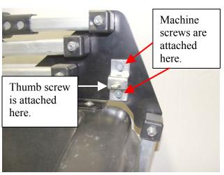
2. Insert rod holder into bracket. Adjust the tension of the rod holder with the thumb screw. The tension at the joint may also be adjusted by tightening or loosening the machine screw. Installation is complete.
