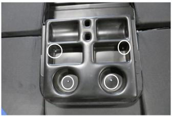
11. Install cots as shown. There is a left and a right one. The shorter support bracket should go to the outside.
