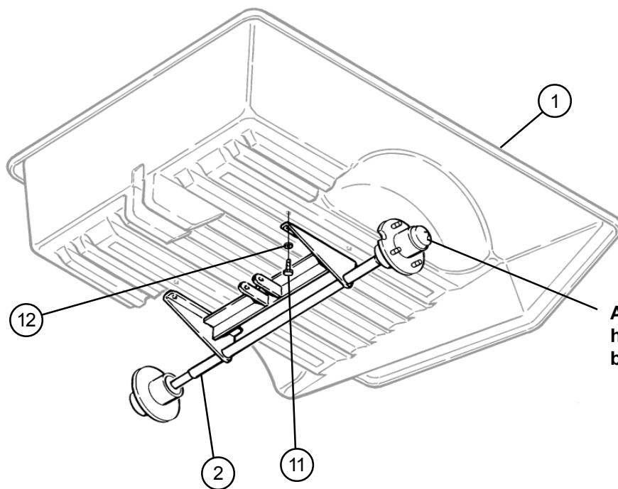
Apply additional grease to the hubs using the grease zerk before using the trailer.
