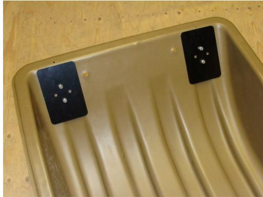
5. Attach the hitch to the sled using the pins that come with the 0400 Otter Sled Hitch.
