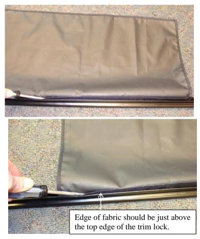
4. Attach trim lock with skirt extension over the existing skirt and shelter fabric and onto the lip of the sled. Secure with the screws that came with the trim lock kit.
