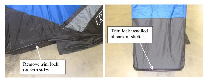
2. Lay trim lock on a flat surface so the opening is facing upward and the outside face is towards you. Lay fabric skirt extension over the top of the trim lock and 1-2 inches from the end as shown. The inside coated surface should face upward.
