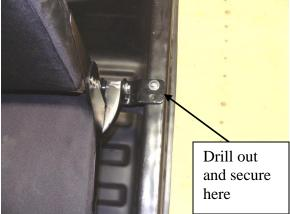
7. Drill out one of the lower holes in the front bracket and secure with the  $\frac{1}{4}$  x 1 bolt, washer and nylock nut. The washer goes on the outside of the sled only. Drill out the second hole and secure. Repeat at the rear of the sled.
