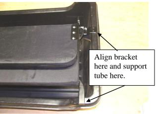
6. After the bench is properly aligned drill out one of the top holes in the front bracket and and secure with the  $\frac{1}{4}$  x 1 bolt, washers and nylock nut. The washers should go on both the top and the bottom. Drill out the second hole and secure. Repeat at the rear of the sled.
