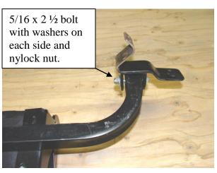
5. Turn bench over from left to right. and align it on the sled as shown. The brackets and the main support tube should line up on the edge of the sled,
