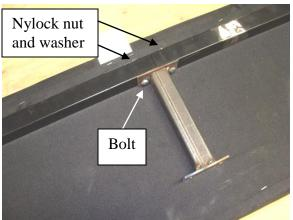
3. Place the second shorter tube on the bench as shown in the picture below. On the left side, line up the inside edge of the tube with the outside edge of the bench. Adjust it as necessary so the holes in the main tube line up with the holes in the center support brace. Attach with the ½ x 2 bolts, washers and nylock nuts. Also attach the tube clamp brackets to the bottom of the bench.
