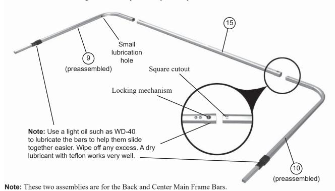
6. Position middle main frame with pivot (Item 15a), left side front elbow and extension (Item 11), and right side front elbow and extension (Item 12) as shown. Align locking mechanism in item 15a with square cutout in items 11 and 12 and slide together until they lock. Lubricate frame bars for best operation as shown in step 5.
