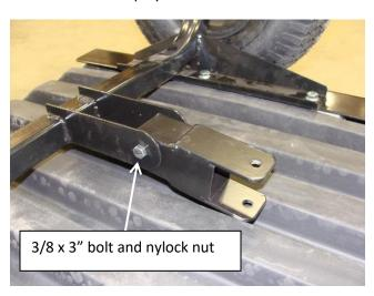
5. Attach tongue to the pivot using the 3/8 x 3" bolt and nylock nut. Tighten the nut enough to hold tongue securely yet allow it to freely move with no excess play.
