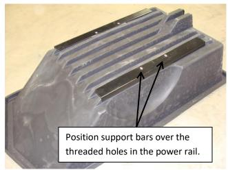
2. Align axle with slots in support bars and threaded holes in the power rails. Tighten securely with the  $7/16 \times 1''$  bolts and lock washers.
