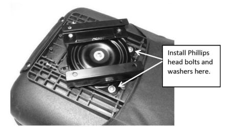
4. Drill out the four pre-marked holes for the seat rail brackets as shown using a 5/16" drill bit. The sled may be tipped upside down to make drilling the holes easier.
