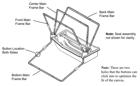
20. Install back adjustable pole (Item 5) as shown first. Install top back support pole (Item 6) as shown next. Install top front support pole (Item 7) as shown next. Install front adjustable support pole (Item 8).
