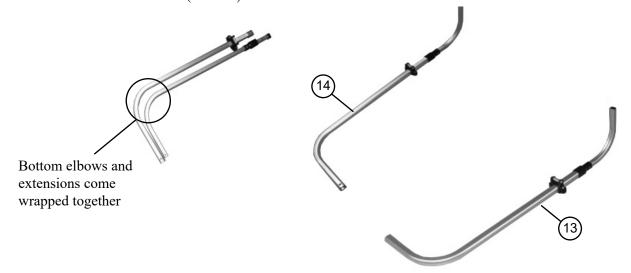
14. Slide middle main frame (Item 15) onto items 13 and 14 assembled in previous procedure and lock together. Lubricate frame bars for best operation as shown in step 11.
