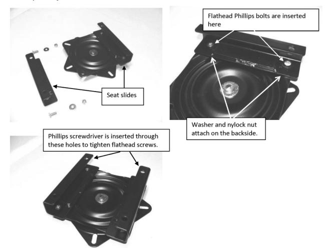
2. Slide brackets and swivel <u>part way</u> onto the plastic base. Adjust the fit to be snug by pressing in on the brackets. However the brackets still need to be able to slide smoothly back and forth on the plastic base. Tighten the bolts securely once the fit is correct.
