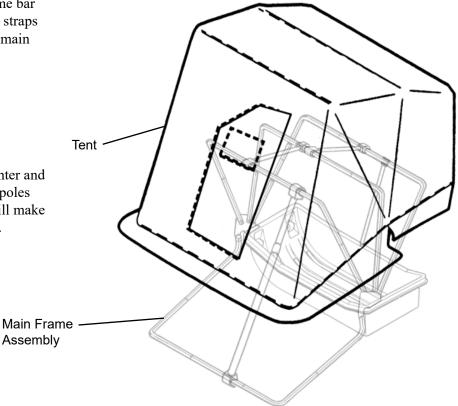
22. Once the canvas is on the frame and the Velcro attached, extend all of the frame bars upward and make sure all of the support poles are installed. Extend the front adjustable support pole so that the fabric in front is snug and not sagging. It will be necessary to loosen the back adjustable pole to achieve this. Once the front is set and the top support poles are in place, the back adjustable pole can be extended until it is snug. Install the plastic trim lock in the positions shown below.
