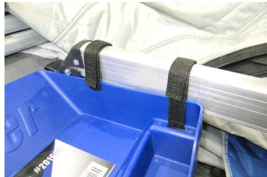
3. Battery straps should be installed as shown. The Velcro should be on the bottom side of the strap when threading it through the slots.
