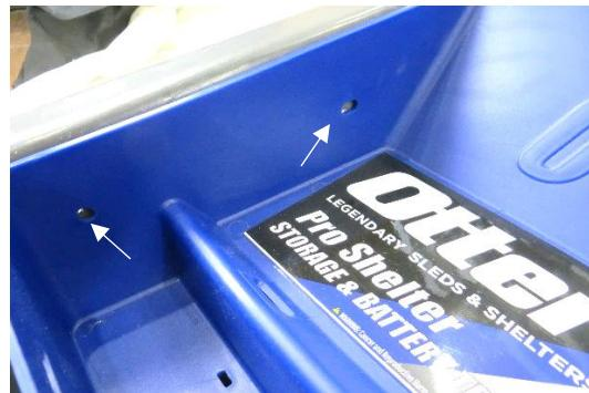
2. Attach with the  $\frac{1}{4}$ " bolts, washers and nylock nuts. Secure tray to the seat rail with the Velcro strips as shown. The tray will be right below the bolt on the seat rail.
