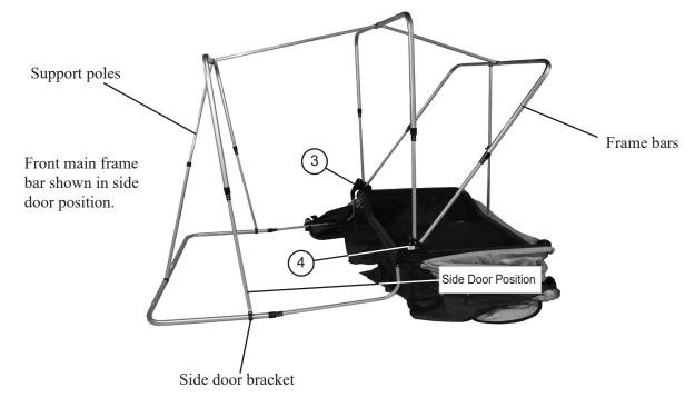
16. Slide the tent over the main frame bar assembly, then fasten the velcro straps on the inside of the tent to each main frame bar.
