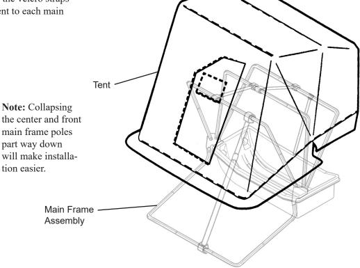
17. Once the canvas is on the frame and the Velcro attached, extend all of the frame bars upward and make sure all of the support poles are installed. Extend the front adjustable support pole so that the fabric in front is snug and not sagging. It will be necessary to loosen the back adjustable pole to achieve this. Once the front is set and the top support poles are in place, the back adjustable pole can be extended until it is snug. Install the plastic trim lock in the positions shown below.
