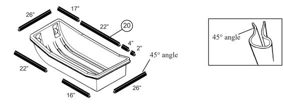
18. On the front of the fishhouse, start in the corners and work inward, snap the plastic trim seal on the canvas tent (Item 2) to the <u>lip</u> edge of the sled (Item 1). The tent (Item 2) will meet in the middle and should be free to open and close so it can be removed.
