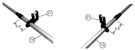
9. Slide middle main frame (Item 15) onto items 13 and 14 assembled in step 7 and lock together. Lubricate frame bars for best operation as shown in step 5.
