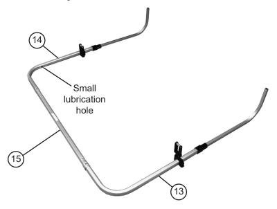
**Note:** This assembly is for the Bottom Main Frame Bar.
